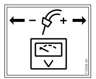
Arc Force/Inductance: This control on the Invertec is disabled in the GTAW mode.
